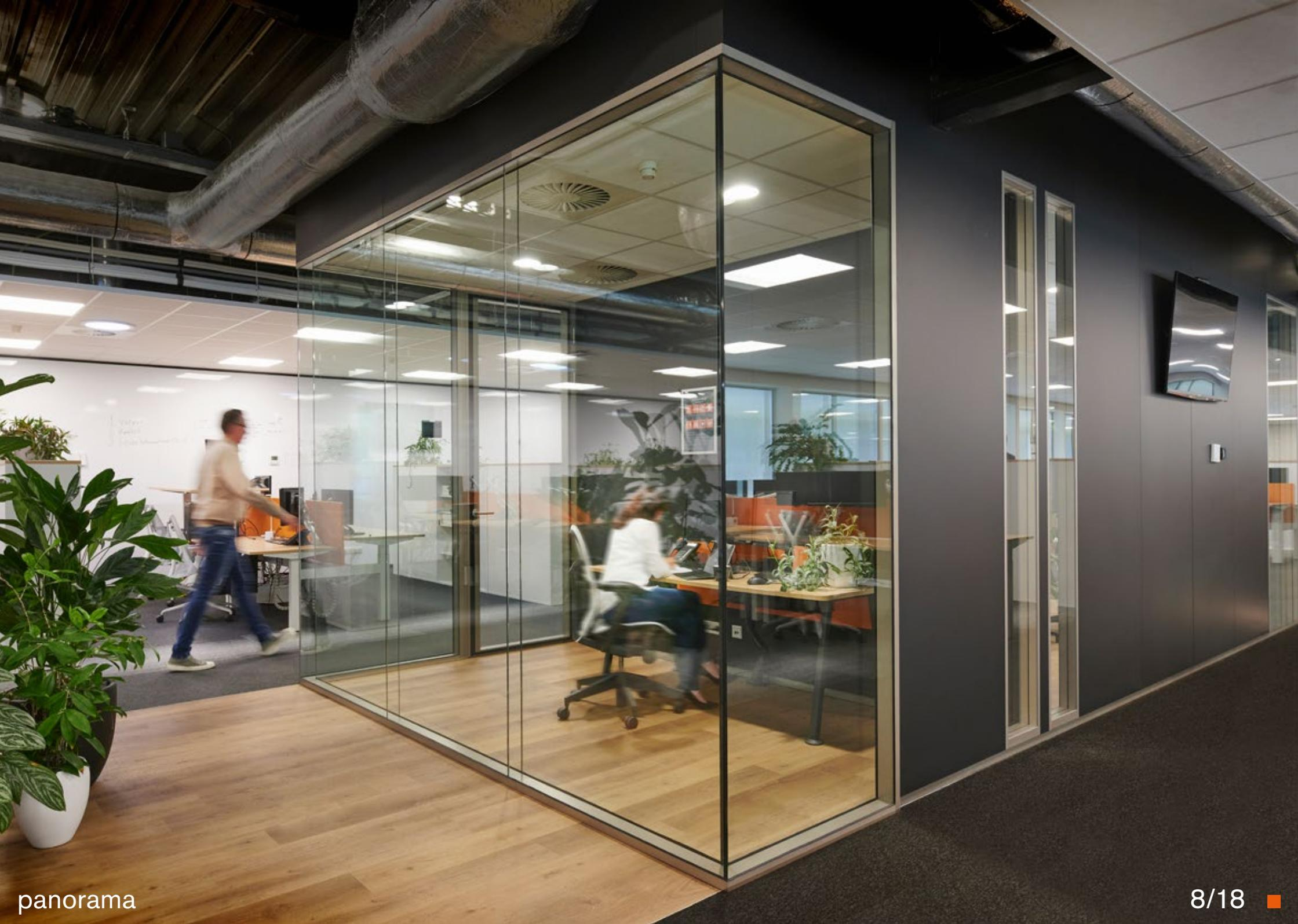
The double-glazed Panorama Slim Tracks system walls allow you to achieve maximum transparency in the interior due to the absence of profiles. The minimalist design of this system creates a super sleek and seamless whole combined with excellent functional performance. No matter what layout you choose, everything is easy to implement and adapt later with a minimum of components. Sustainable and permanently flexible!
